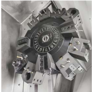
H70MH SAUTER(GPM) 12T powered tool turret
