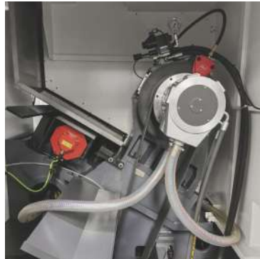
H70MH CS axes with hydraulic brake
