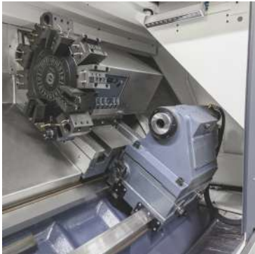
X Z axes and tailstock BOX guideway
